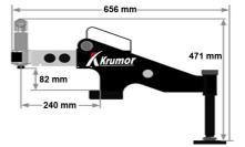
Minimum applicable Bolt Hole Diameter 35.5 mm (1.40")
