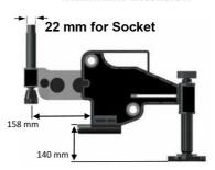
Minimum applicable Bolt Hole Diameter 25mm (1.0")
